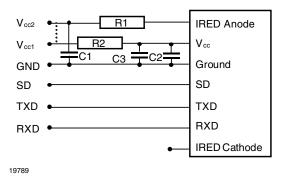
Fig. 1 - Recommended Application Circuit
