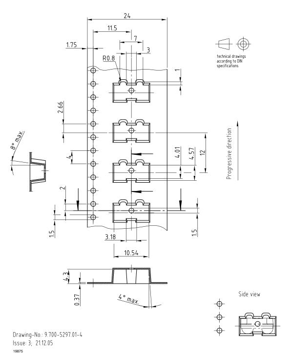
Fig. 9 - Tape Drawing, TFDU6103 for Side View Mounting, Tolerance  $\pm$  0.1 mm
