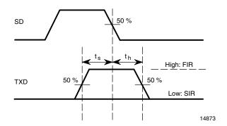
Fig. 2 - Mode Switching Timing Diagram
