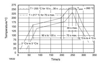
Fig. 4 - Solder Profile, RSS Recommendation
