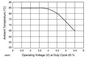
Fig. 6 - Temperature Derating Diagram
