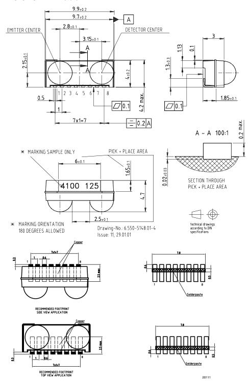
Fig. 7 - Package Drawing and Solder Footprints for Top and Side View Mounting TFDU6103, Tolerance ± 0.2 mm if not otherwise mentioned
