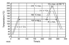
Fig. 3 - Recommended Solder Profile for Sn/Pb soldering
