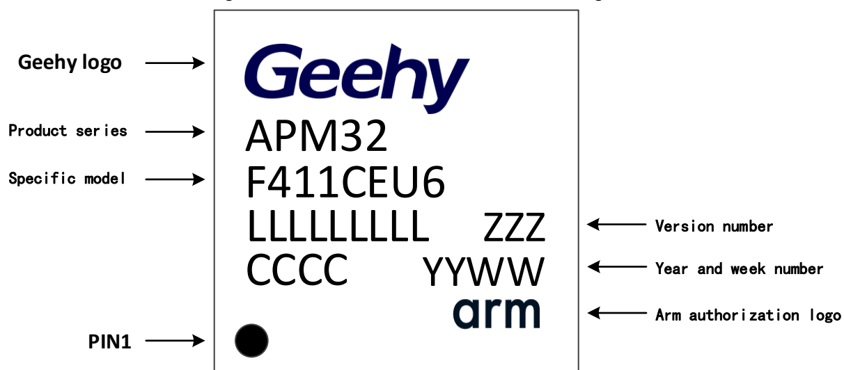
Figure 28 QFN448 - 48 Pins, 10 x 10mm Diagram
